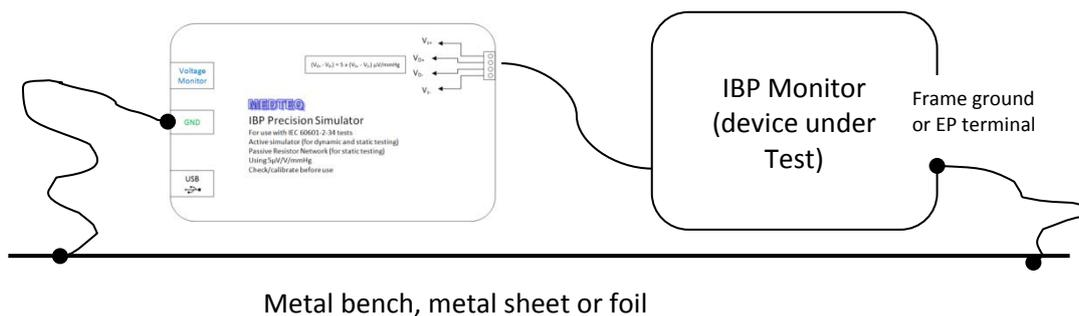
With this set up, turn the IBP monitor on and confirm that the level of noise is acceptable for tests. For most tests, this set up is satisfactory without any special efforts.
