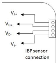
Users can attach additional leads to the V<sub>D+</sub> and V<sub>D-</sub> terminals to monitor the applied differential voltage (V<sub>D</sub>) directly. This should be zeroed as described in 4.3.
