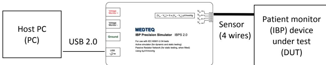
The host PC provides commands to the USB Module to set up relays, or output voltage depending on the mode selected by the user.
