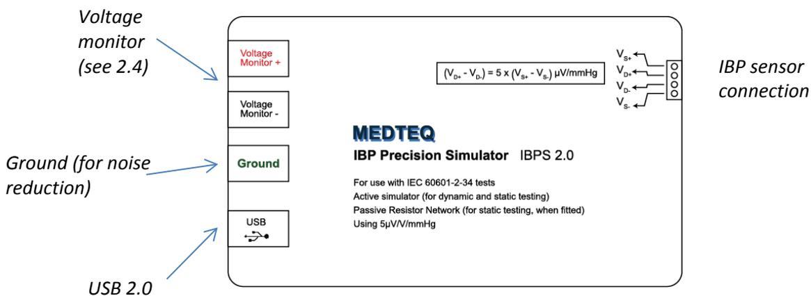
**Important note:** this system assumes a floating (isolated) measurement circuit in the IBP monitor (i.e. Type CF patient isolation). If the circuit is not isolated, and the system grounds are common, there may be sufficient noise to introduce errors.
